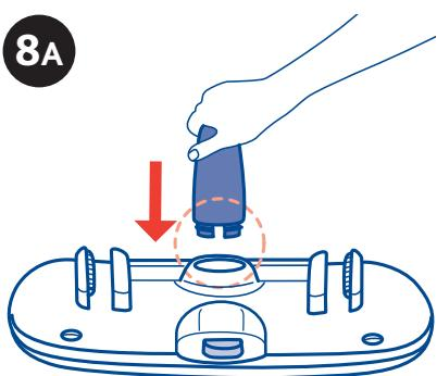
8. Fit the rigid crotch strap to the tray (diagram 8A, diagram 8B). The design of the crotch strap attachment only allows one type of assembly operation. The tray can now be fitted to the Highchair.
