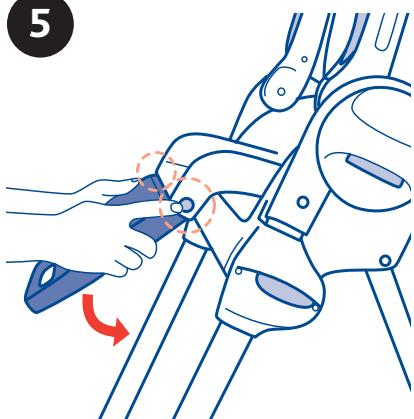
5. Press the side adjustment buttons and lower the leg rest in a vertical position (diagram 5).
