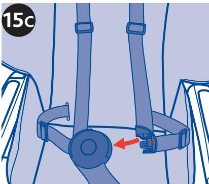
15C. Insert the waist belt clip into the crotch strap buckle, it will click into place. The harness straps can be adjusted to better fit your child (diagram 15D).
