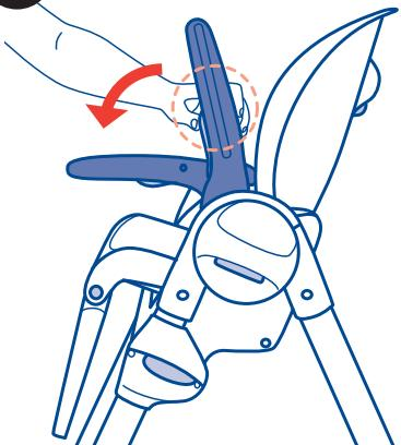
7. Lower the armrests by pressing the two buttons located at the bottom of the armrests (diagram 7).
