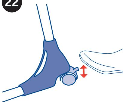
22. To apply the brakes, lower the wheels locking levers. To release the brakes raise the wheels locking levers (diagram 22).
