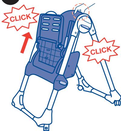
3. Raise the seat by holding the upper part of the backrest and pull it upward, until the desired height is reached (diagram 3). The Highchair can be adjusted to 7 height positions.
