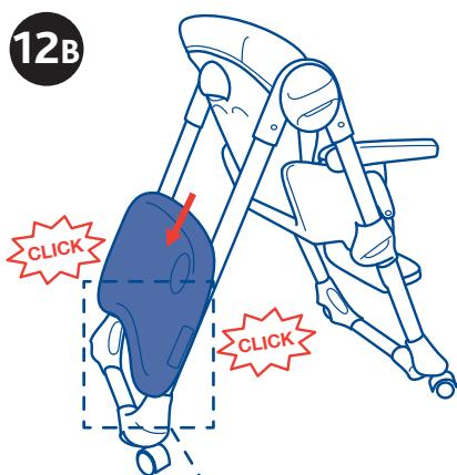
12. When not in use, the tray can be stored on the rear legs of the frame by using the rear leg slots as shown in 12A. With the tray resting against the rear legs, above the slots and locking guides on the inside of the rear legs. Allow the tray to slide down the legs and lock into rear leg slots (diagram 12B). To release the tray press the locking button and remove from the legs.
