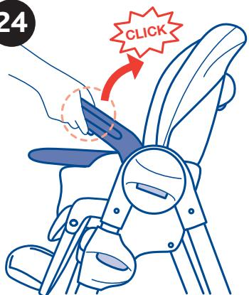
24. Raise the armrest in a vertical direction by pressing the buttons located on the lower part of the arm rests, until an audible click is heard (diagram 24).
