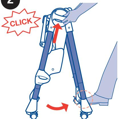
2. Stand at the back of the highchair and hold the two side joints, then press the open/close buttons. At the same time, open the Highchair legs using your foot, until an audible click is heard, signalling that the legs are locked in the open position (diagram 2).
